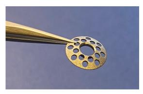
• The back plate (8.5 mm diameter) with a central hole, and 16 holes (1.2 mm each)
